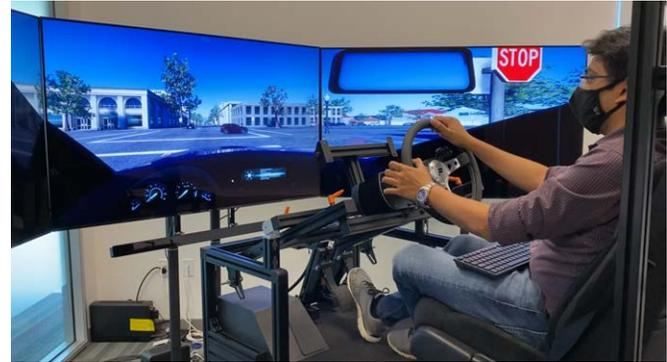
Fig. 1: Our driving simulator is composed of a steering wheel and two pedals mounted on a cockpit, and three 55-inch displays showing the front and side views of the virtual environment.
